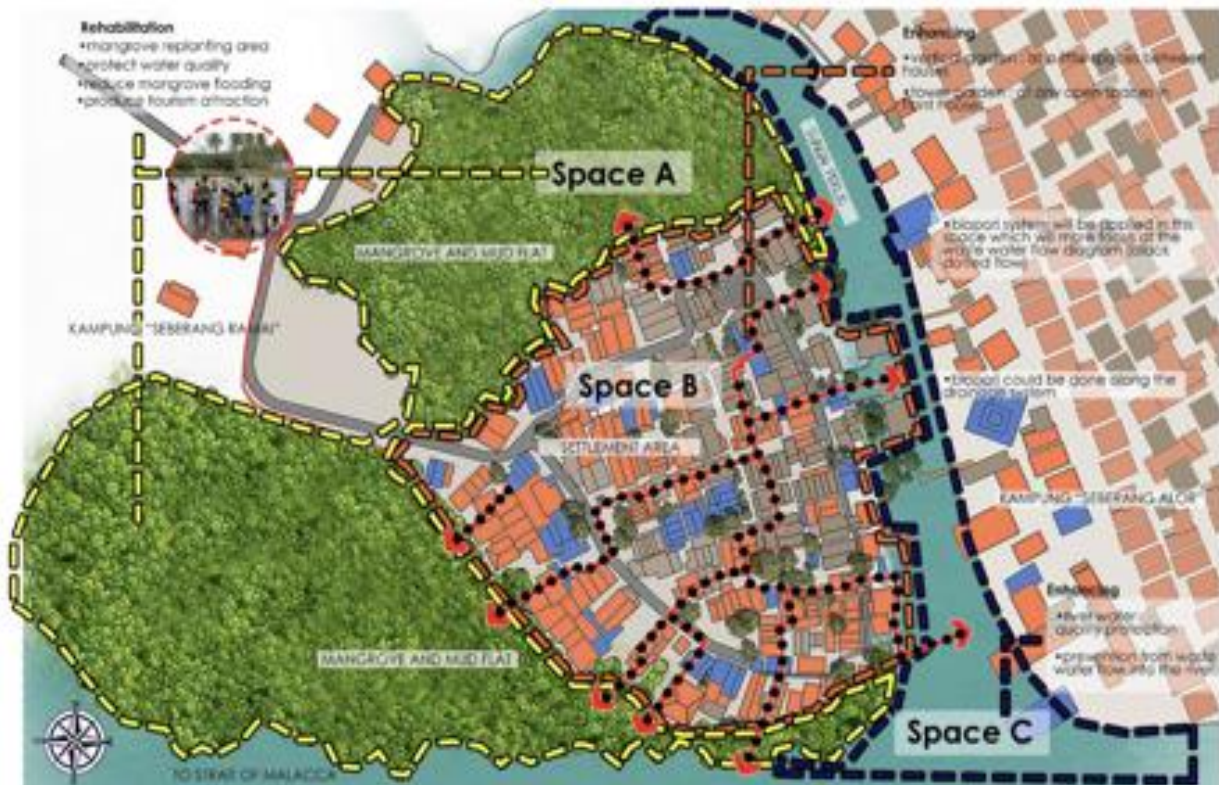
Figure 1: Space-A to restore and rehabilitate with replanting mangrove trees; Space-B proposed with green area, bio Pori system, rain-barrel, and porous roadway
